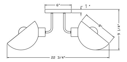
Each metal shade rotates allowing various positions
